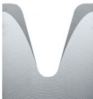
Bottom tool with WILA's proprietary CNC-Deephartening™ process applied.
