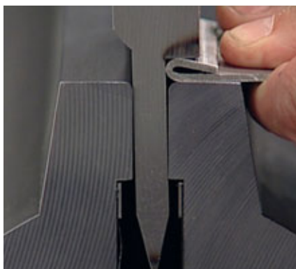
Pre-bend and flattening in the same tool.
